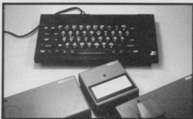
▲ The starter pack: Red Leader, the control centre; Red Two, the infra-red detector; and Red One, power control
